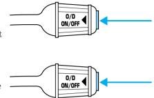
When you shut off and re-start your vehicle, the transmission will automatically return to normal 0 (Overdrive) mode.
